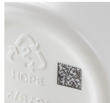
The Videojet 7810 laser system leverages Ultraviolet wavelengths to create permanent, high resolution codes on HDPE packaging
